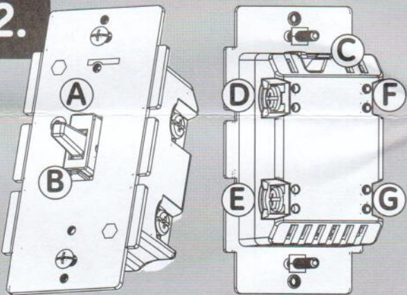
**A. UP** — Press UP & release to turn Dimmer on, press up & hold increases brightness!
