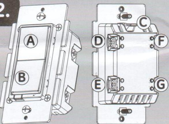
**A. Top Rocker** — (Press & release to turn Dimmer on, press & hold increases brightness)
